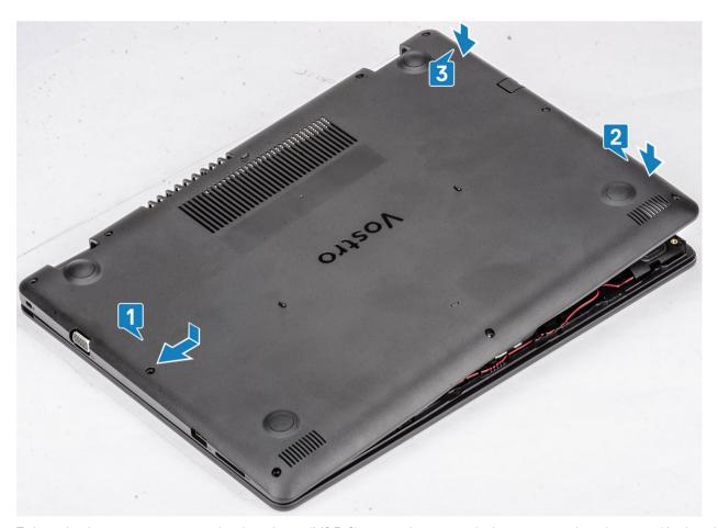
3 Tighten the three captive screws and replace the six (M2.5x6) screws that secure the base cover to the palmrest and keyboard assembly [1, 2].
