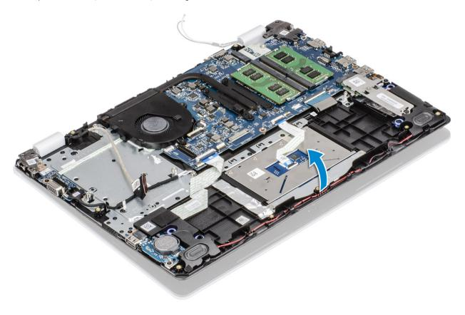
6 Slide and remove the palmrest and keyboard assembly off the display assembly.
