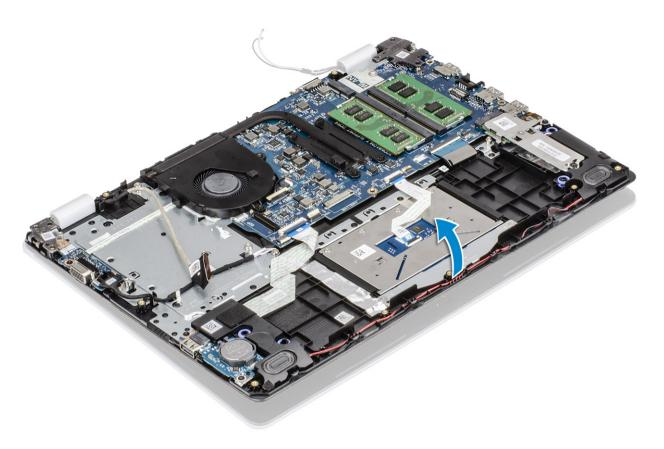
Replace the four (M2.5x6) screws that secure the left and right hinges to the system board, and palmrest and keyboard assembly.
